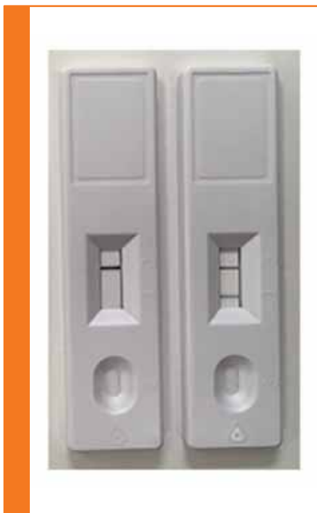
Figure 3. Lateral flow assay to detect NR2 antibody in buffer within 2 minutes: negative control (left) and positive sample (right).
